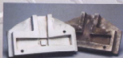
*Baked-on deposits are removed quickly without harmful abrasives or added media contaminants.*
